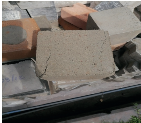
Figure 5.4: Compressive Strength Test Performed at the Materials Testing Laboratory
