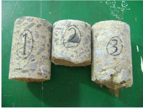
Figure 01: Concrete Core Samples
